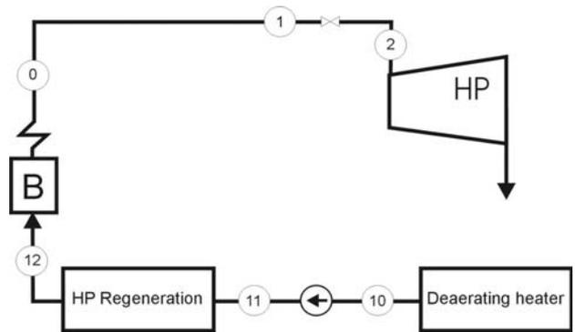
Fig. 4. Simplified scheme of the turbine heating system
