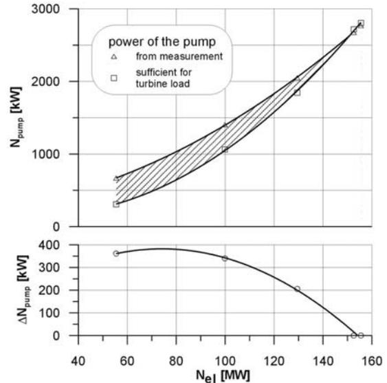
Fig. 10 Power change of the feed water pump
