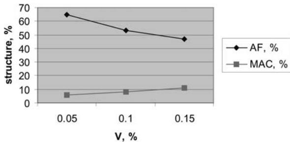
Fig. 6. Metallographical structure with V in MWD
