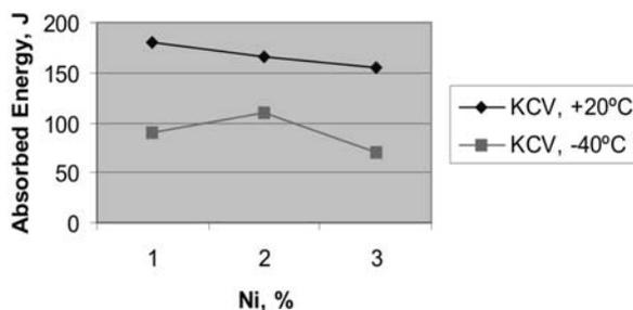
Fig. 4. Relations between the amount of Ni in MWD and the impact toughness of MWD
