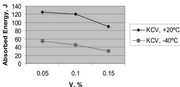
Fig. 2. Relations between the amount of V in MWD and the impact toughness of MWD
