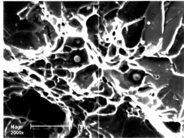
Fig. 9. Fracture surface of metal weld deposit
