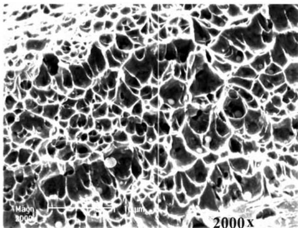
Fig. 8. Fracture surface of metal weld deposit
