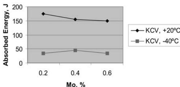
Fig. 5. Relations between the amount of Mo in MWD in MWD and the impact toughness of MWD
