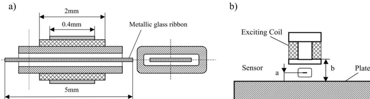
Fig. 3. a) Fluxset sensor geometry b) Probe set-up
