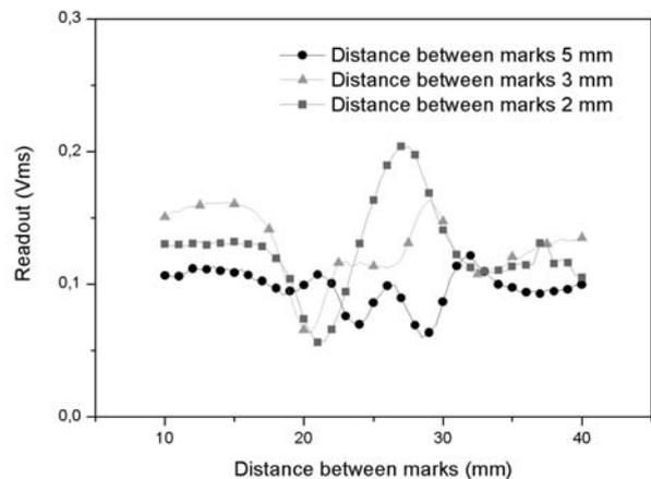
Fig. 8. The result of readout on laser scribed steel sheets. The applied laser density was 190 W/mm<sup>2</sup> (150 W)
