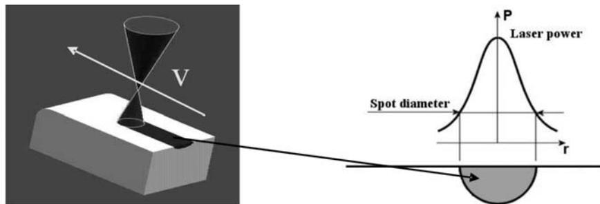
Fig. 2. Process of laser scribing and modal structure
