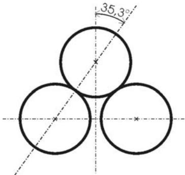
Fig. 1. Geometry of loaded balls in sliding contact
