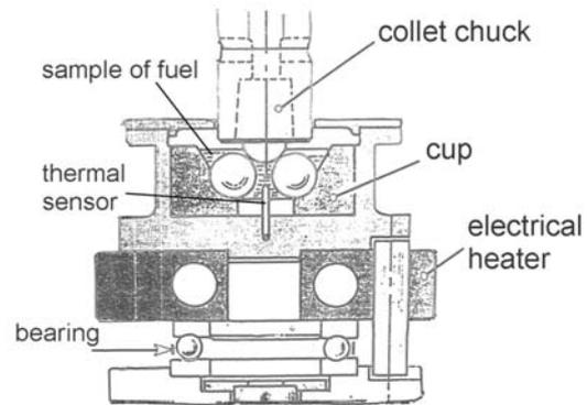
Fig.2 Configuration of the test assemblies
