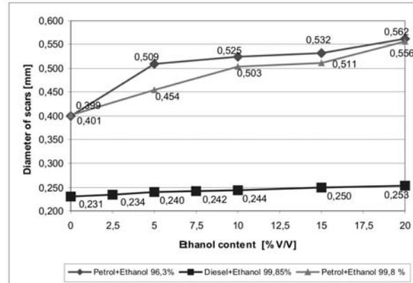
Fig.4. Lubricity of tested fuels
