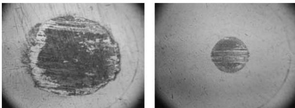
Fig.3. Friction mark on balls with fuel diesel + ethanol on left and petrol + ethanol on right
