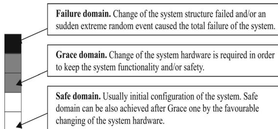
Fig. 2. Three possible states of the process variable in Dynamic Reliability approach
