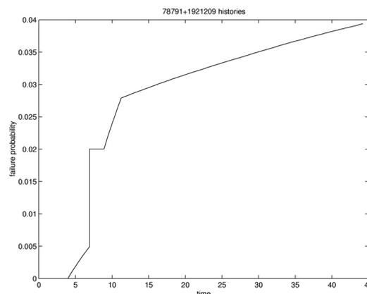
Fig. 4. Evolution with time of  $PL(t)$  for  $\lambda = 4 \cdot 10^{-2}$  computed via direct Monte Carlo simulation
