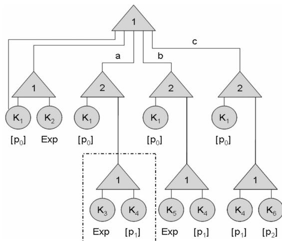
Fig. 3. The time dependent acyclic graph representation of the dynamic reliability test-case. Symbols  $a, b, c$  denotes the following time intervals:  $a = (8.892; 11.247)$ ,  $b = (11.247; 44.205)$ ,  $c = (44.205; \infty)$
