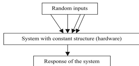
*Fig. 1. Traditional Probabilistic Safety Assessment (PSA). Stochastic character of system inputs is described by random variables. The output of PSA is a response of the system, for instance probability of failure. In contrast of Dynamic Reliability approach, methodology of PSA assumes that the structure of the system is constant, non-changing, stable*
