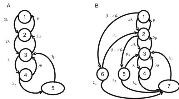
Fig. 1. State space diagram for auxiliary system operating in mode 1 (A) and in mode 2 (B).
