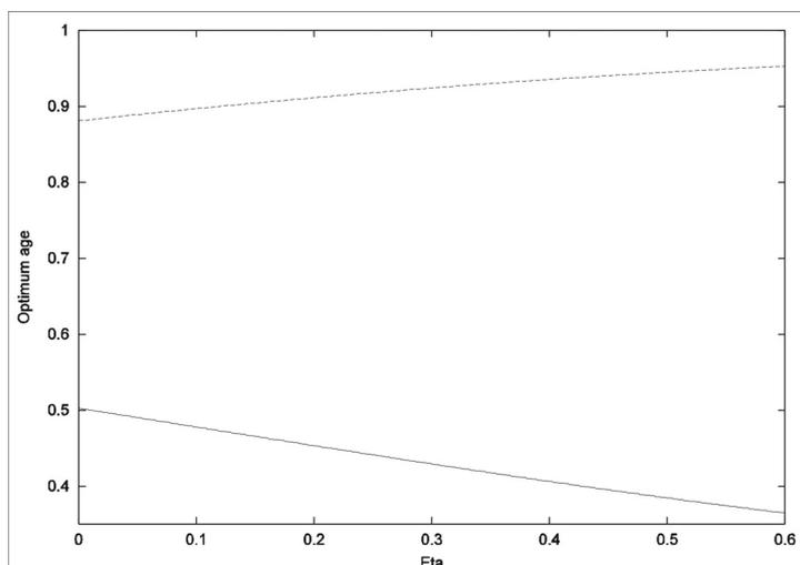
Fig. 1. Age based replacement with a Weibull distribution of scale parameter 1, shape parameter 3, replacement cost  $c_s = 1$ , failure cost  $c_f = 5$ . The solid line shows the variation of optimum age at replacement with the risk-aversion parameter  $\eta$ , and the dotted line the survival function
